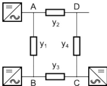
A network with one mesh of interconnected VSI, coupled by the line impedances will be set up.
