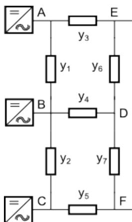
A complex network with two meshes, three VSI and two nodes with connected loads will be set up.
