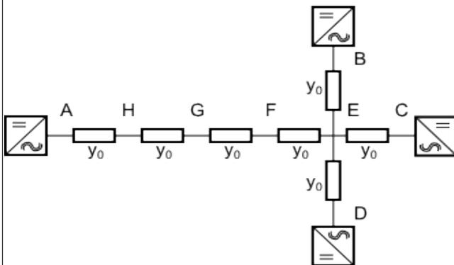
The proposed setup will be used to investigate the frequencies, measured by the PLLs of the VSI in the nodes B,C and D upon a frequency change of the VSI in node A.
