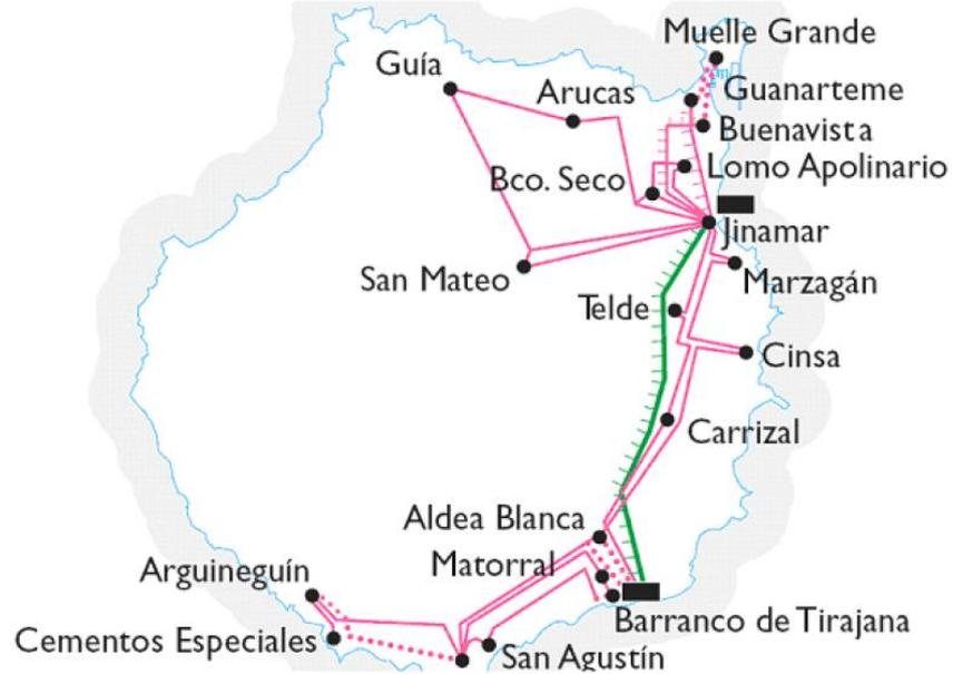
*Figure 1.* Gran Canaria Island's electrical grid, high voltage layout (provided by Red Eléctrica España).
